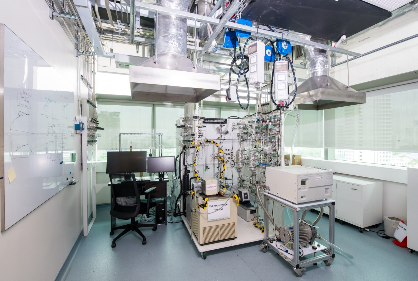
Fig. 1.15: Vacuum Swing Adsorption pilot plant rig.
