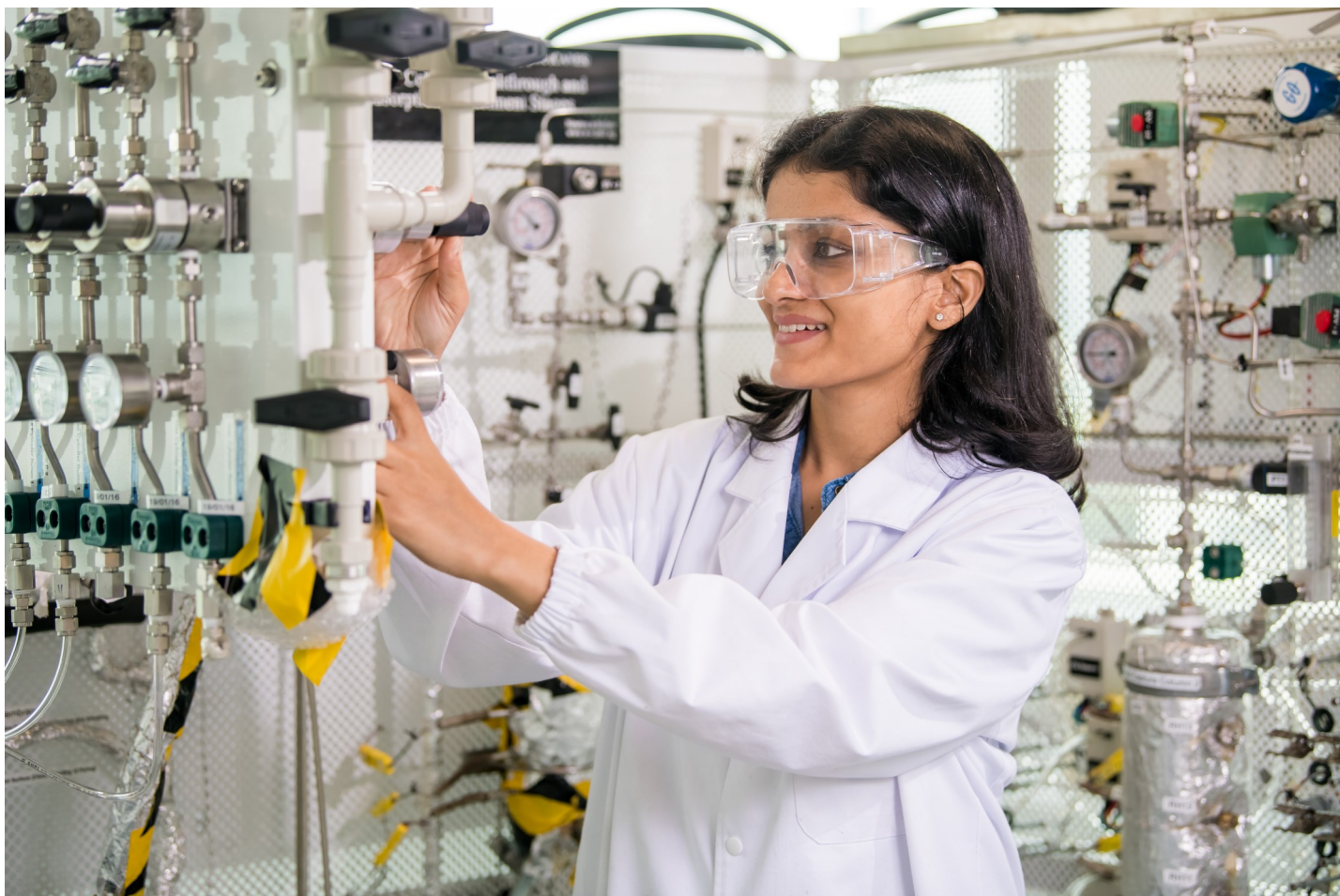
Perna Goyal (PhD student, NUS, IRP1) works on the Vacuum Swing Adsorption pilot plant rig.
