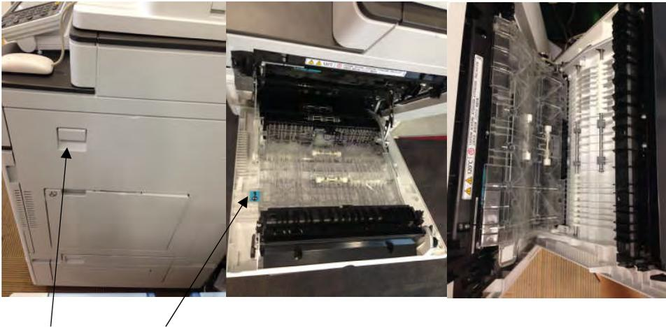
For clearing of paper misfed, please open the handle on the right hand side and remove the paper accordingly. Use the blue tap to lift up to clear the paper that is jammed.
