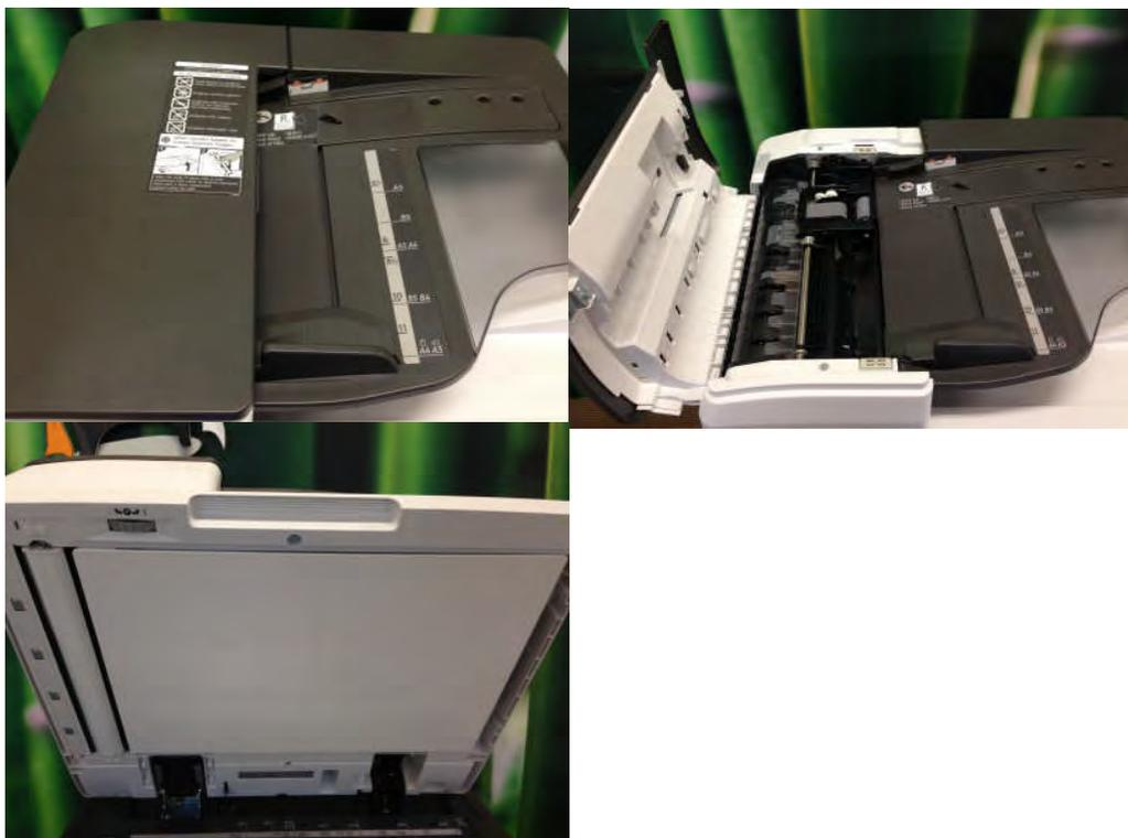
If you encounter paper misfed on the top feeder, please lift up the handle of the feeder and remove the paper.
